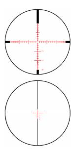
• The reticle is positioned in the front focal plane and his type is MP8 – adapted for MOA.
